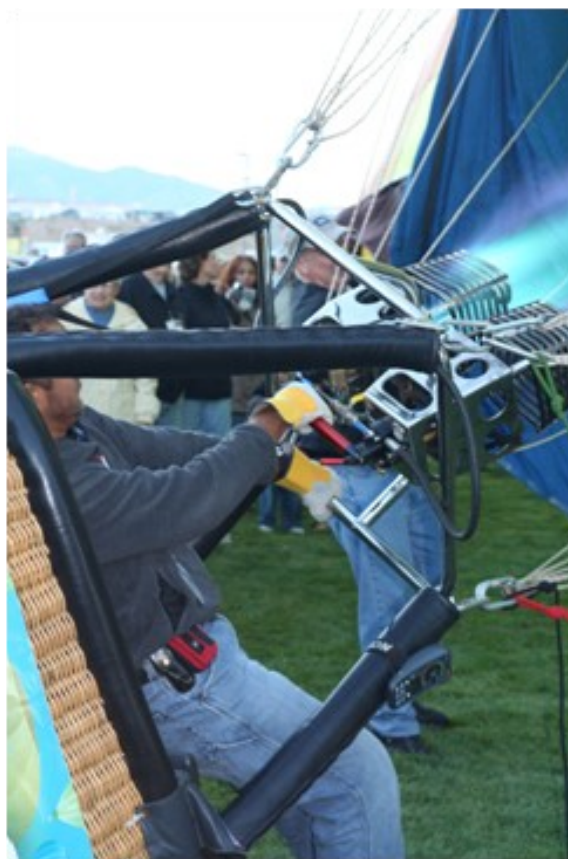
The propane burners heat the air.
